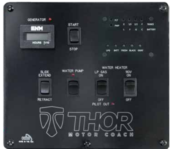
Typical Monitor Panel
